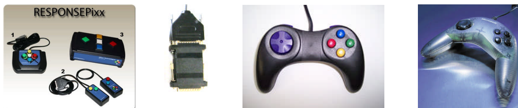
Figure 2-6: VPixx Button Boxes (left), VPixx Button Box Parallel Port Pin Adapter, modified Gravis Destroyer gamepad, and Microsoft USB Sidewinder gamepad (right)
