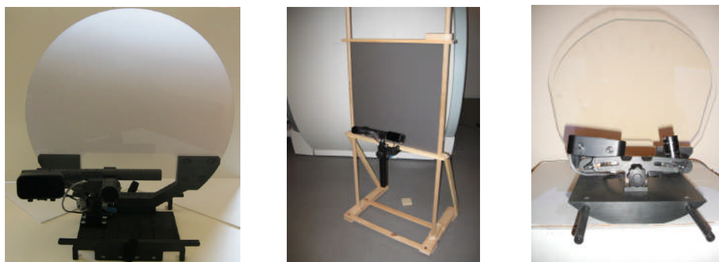
Figure 7-11: Tray Mount with optional screen for Siemens family of scanners (left), Screen Mount (middle), and Siemens Allegra short bore mount (right)
