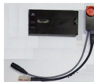
Figure 2-1: The Standard Camera (left) and Fiber Optic Camera Base Box and Camera Head (right)
