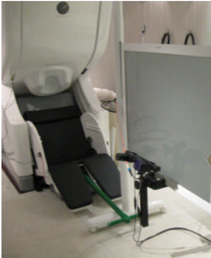
Figure 7-10: Screen Mount used in conjunction with the Elekta Neuromag screen (left) and a custom-built wood-frame screen (right)
