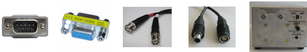
Figure 7-7: Male DB-9 connector (left-to-right), gender changer with female connector showing, BNC connectors, LEMO connectors, and Battery System
