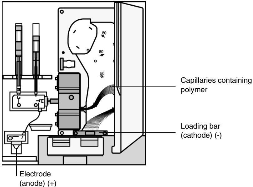
**Description** During electrophoresis, a high voltage is applied between the loading bar (cathode) and the electrode located on the lower polymer block (anode). The voltage drives the movement of negatively charged DNA fragments through the polymer in the capillaries towards the anode. From the anode, the current flows back in electrical wires through the power supply to the cathode to complete the circuit.
