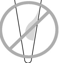
The sample lies on the side wall because the plate was not centrifuged. |
