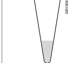
The sample is positioned correctly in the bottom of the well. |
