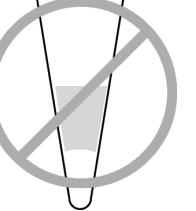
An air bubble lies at the bottom of the well because the plate was not: <ul style="list-style-type: none"><li>◆ Centrifuged with enough force, or</li><li>◆ Centrifuged for enough time</li></ul> |
