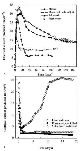
**Figure 1.** (A) Examples of current production by laboratory fuel cells constructed using sediments from three different sources under identical loads (1000 ohms), and effect of amending the marine sediments with 100  $\mu$ M AQDS. (B) Effect of sterilization on current production in laboratory marine sediment fuel cells.
