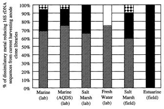
**Figure 2.** Relative proportions of dissimilatory metal reducing 16S rRNA gene sequences associated with the current harvesting anode from five separate fuel cells. Hashed lines: *Geobacteraceae*; black: *Desulfobulbus/Desulfocapsa* species; diamond pattern: other sulfate reducing δ-Proteobacteria; white: *Geothrix* species.
