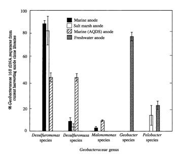
**Figure 4.** Relative proportions of *Geobacteraceae* 16S rRNA gene sequences associated with the current harvesting anode from four separate laboratory fuel cells.
