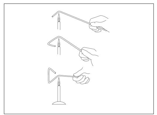
Figure 1.1.3 Making a spreader.
