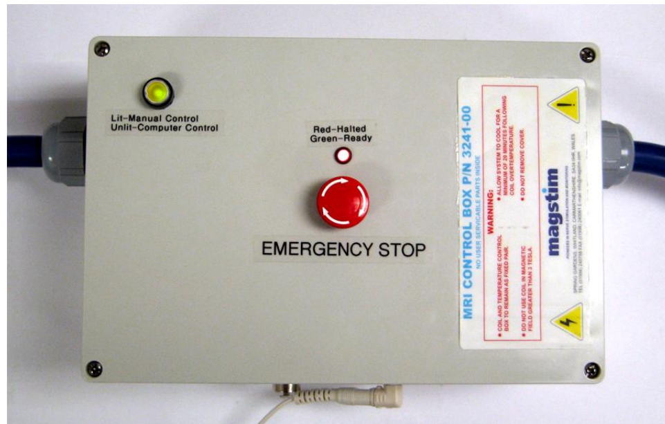
Figure 5 The new coil control box with the pneumatic foot pedal removed and the new safety switch installed. This box also contains added noise elimination circuitry that is described below. The button in the top left corner switches between manual and computer control; manual control is useful for debugging and experiments outside the scanner. The large red button will immediately disconnect the coil when struck, this may be necessary if the subject has a seizure.
