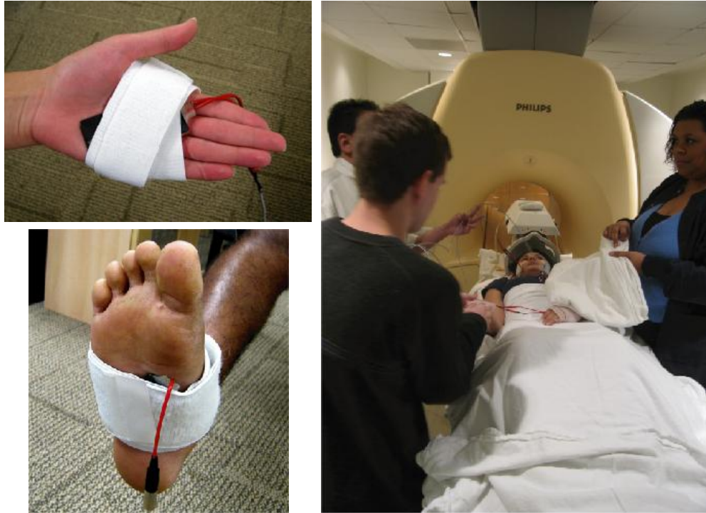
Figure 2 (Left) The piezoelectric bending actuators are attached to a subject's hands and feet using elastic bandage wrap. (Right) Six piezoelectric bending actuators are being attached to a subject's hands, feet, and face.
