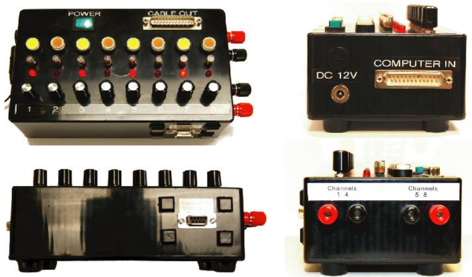
Figure 5 The control box. The top view shows activation buttons, attenuating potentiometers, and protection fuses. The front and rear views on the right show the computer and signal input.
