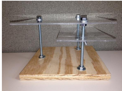
Figure 6B Large plexiglass resting on and secured by washers and nuts
