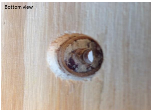
Figure 5A Bottom of board showing depth of countersink hole
