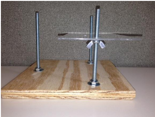
Figure 6A Small plexiglass resting on washers and wingnuts
