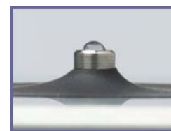
Properly Conditioned Pedestal-water “Beads up”
