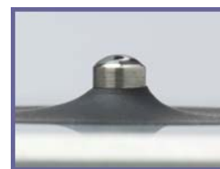
Un-conditioned Pedestal- water “Flattens out”
