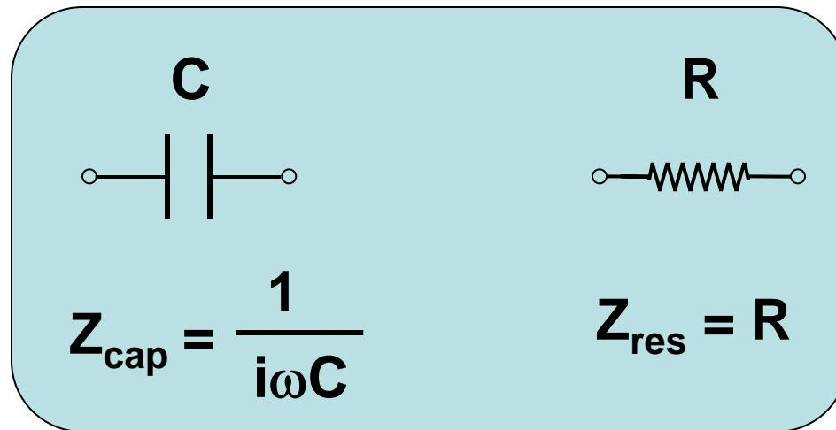
Differential Equation  $\rightarrow$  Algebraic Equation  $\rightarrow$  Impedance Model
