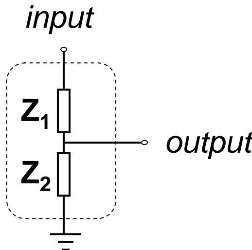
Input impedance:  $Z_{\text{input}} = Z_1 + Z_2$
