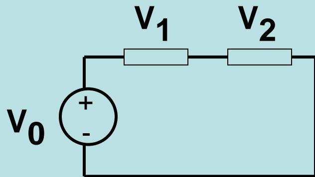
$$V_0 + V_1 + V_2 = 0$$
