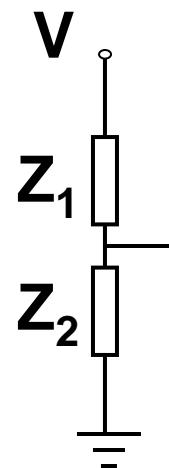
$$V_{\text{out}} = V \frac{Z_2}{Z_1 + Z_2}$$
