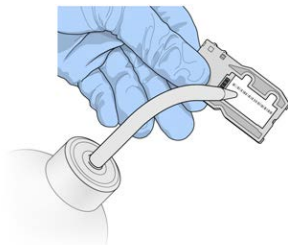
Figure 33 Rinse Flow Cell
