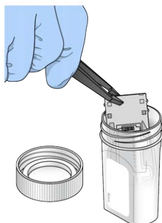
Figure 32 Remove Flow Cell
