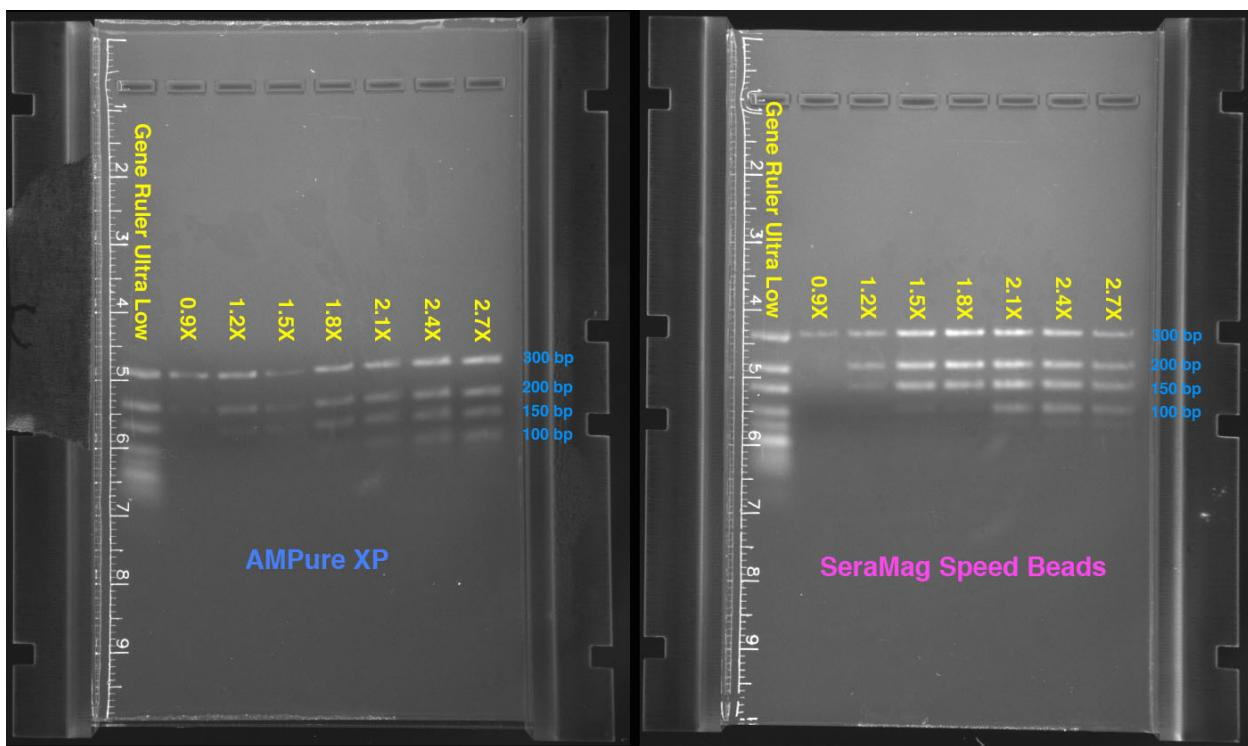
As you can see, the volume of AMPure or SeraPure controls the size of fragments recovered. More specifically, it is the ratio of PEG solution used to the volume of the DNA in solution which makes the difference, not the count of beads in solution (provided they are above the minimum level). This is what makes it possible to do “double-SPRI” size selection.
