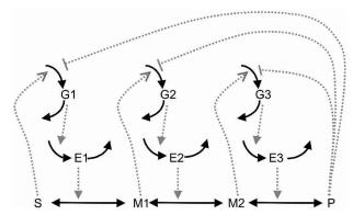
**Figure 1** The model metabolic pathway used in these studies. Solid arrows represent mass flow, dashed arrows represent kinetic regulation; arrow ends represent activation, blunt ends inhibition. S and P are the pathway substrate and product and are held at constant concentrations;  $M_1$  and  $M_2$  are intermediate metabolites of the pathway;  $E_1$ ,  $E_2$ , and  $E_3$  are the enzymes;  $G_1$ ,  $G_2$ , and  $G_3$  are the mRNA species for the enzymes.
